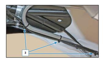
Slide the cables (4) of the direction indicators out from the hole in the mud guard.
