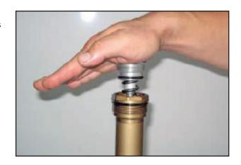
Block the orthogonal external area of the cartridge assy.
