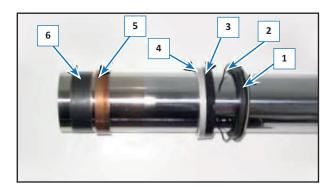
Mount the metal bush and the washer on the external pipe, inserting them into the housing with the aid of a guide.
