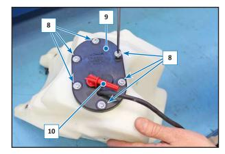
Check that the gasket (11) is not ruined and is positioned correctly, then tighten the screws (8) gradually cross-wise, until they are fully home on the plastic of the pump (9) compressing the gasket (11). At this point, tighten them by 1/2 turn, 1 turn max.
