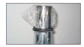
NOTE: Apply grease to the edge of the sealing ring.
