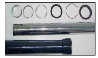
Check that the internal rod has no distortions or damage.
