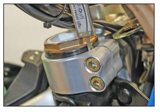
NOTE: Normally the distance is approx. 13 mm on the first reference notch of the rod.
