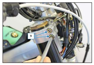
NOTE: On re-mounting, position the rods on the upper steering plate at the measurement obtained and then tighten the screws (9) with a torque of 20 Nm/ 2.0 kgm/ 14.75 ft/lb and the screws (10) with a torque of 15 Nm/ 1.5 kgm/ 11.06 ft/lb.
