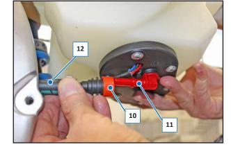
NOTE: Re-mount everything proceeding in reverse order to disassembly, paying attention to wrap the sheath (8) around the fuel hose (12) and the pump electric connection cable.
