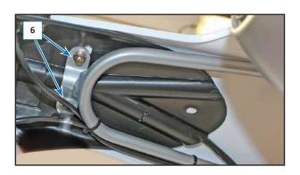
Slide the cable (7) out from the hole in the mud guard.
