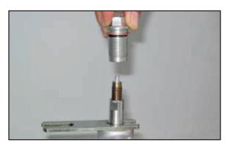
Tighten the adjustment screw to the stop position.
