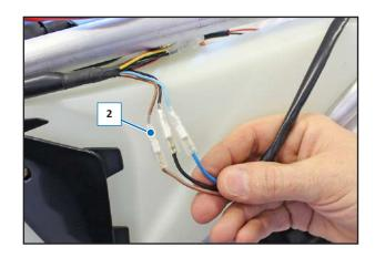
Disconnect the wires (3) of the rear direction indicators.
