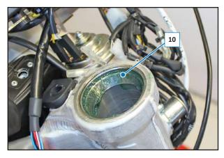
NOTE: On re-mounting, clean the inside of the steering head and the steering pin well. Insert the bearing housing using a punch. Remount the bearings, greasing both the housing and the bearings.
