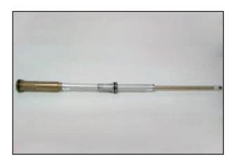
Remove the foot valve unit from the cartridge assy.
