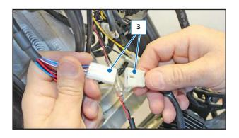
Disconnect the connectors (4) of the front direction indicators.
