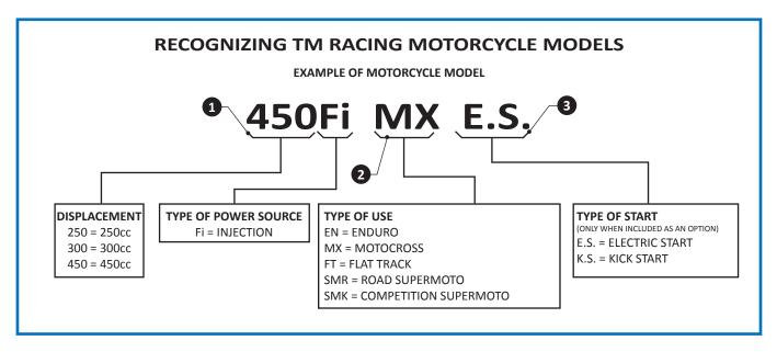
The displacement, type of power source and type of use define the model of motorcycle and engine of each TM Racing bike.
