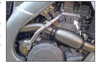
Starting from the highest position, push the starter all the way down with fast, continuous movements.
