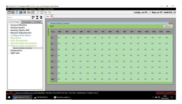
• Injection auxiliary correction: the value 1000 indicates the quantity of default fuel. It is possible to grease up to 30% (1300) and lean up to 30% (0.700); otherwise, it is possible to vary the engine revolutions threshold and throttle % by changing the value on the main column. The modified values remain highlighted with a different colour.
